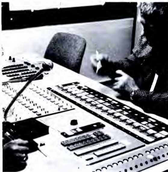
Delegation switcher in VTR control room is tagged with colored stickers, the different colors representing different sporting events. This was to avoid confusion in assigning any of the 17 AVR-1's in the VTR pool.
