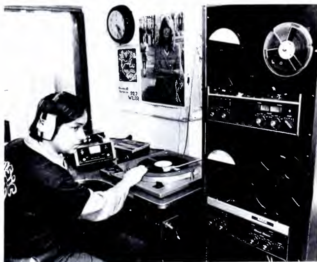
WLIR's chief engineer, George Sullivan, cues up a disc for recording on one of the Revox A77's used for origination of most music programs at the Long Island FM station.
