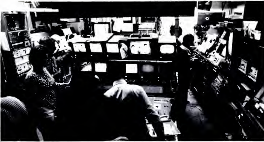
BBC switching and VTR room containing four VR-2000's equipped with Conrac monitors and a portable VR-3000 for field work.
